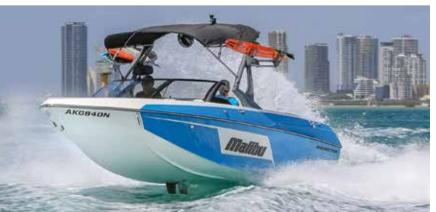
that help keep a perfect line, and reverse chines that help lift the hull at ski speeds to create soft, passable wakes for tournament-quality slalom skiing.
